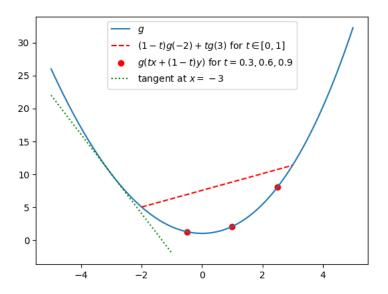
Convex functions are often described as having the shape of a smile. The key point is that the red dots, corresponding to the left hand side of (6.4), sit below the red line, corresponding to the right hand side of (6.4). Here we have shown (6.4) for x = -2 and y = 3, on the convex function  $f(x) = 1 + x^2 + \frac{1}{20} \max(0, x^3)$ . The tangent line at -3 is shown in green. Note that f sits above its own tangent lines.
